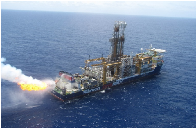
The Stena DrillMAX is a Harsh Environment dynamically positioned DP Class 3 drillship capable of drilling in water depths up to 10,000ft.
