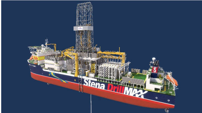
The Stena DrillMAX is a Harsh Environment dynamically positioned DP Class 3 drillship capable of drilling in water depths up to 10,000ft.
